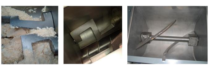
Amalgamator in mixing is used to mix all the liquid and solid ingredients to obtain a raw material that will be refined in the subsequent machines.
