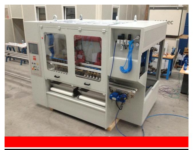
Multi flash stamper (MFS model) in shaping process is used to create finished soaps from a cut bar through a flashstamping process. Flashing from the dies falls on the flat belt and it's taken out of the machine through the back wall making an easier recycle line.
