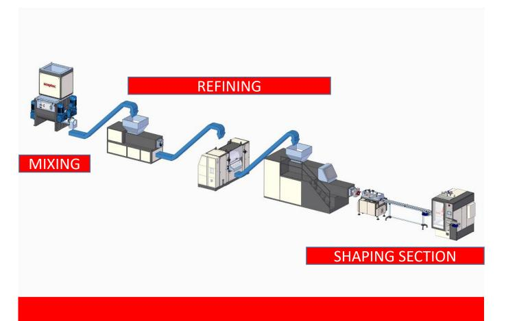
Any finishing line has to put together all the elements of the recipe and shape the product into a form (tablet) for final use. So, every line begins with Dosing&Mixing section, composed of Mixer and eventual dosing group and ends with Shaping section.
