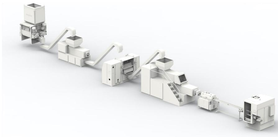
Finishing Line is a name given to an assembly of machines that are working the soap in order to produce a finished product (soap bar) of desired apperance and quality.
