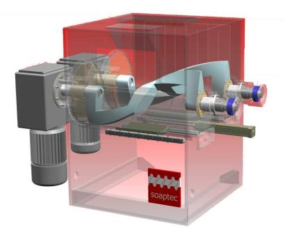
Double arm sigma mixer in mixing and refining is used to mix all the liquid and solid ingredients to obtain a raw material that will be refined in the subsequent machines. The double arm mixer has two big sigma blades and can be provided with choppers. It's designed to coat and brake the pellets for an intensive mixing.
